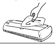
**Caution:** Do not spray cleaning fluid directly on the scan window, transparencies, or scanner surface.
