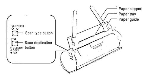
Scan type button Press once to toggle between text and photo mode.
